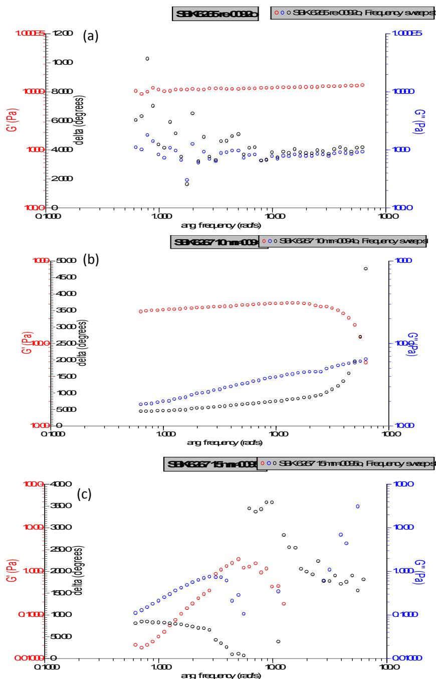
**Fig S1.** Frequency sweep at a fixed oscillatory stress of 1.0 Pa for (5 mM: 15 mM) Tb/NaC gel with a) 0 mM NaF; b) 10 mM NaF; c) 15 mM NaF.
