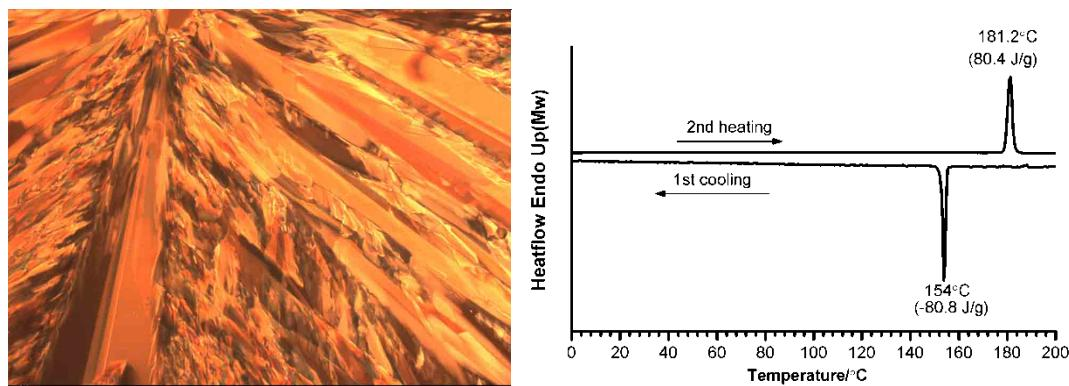
**ESI Fig. 27** Crystalline texture observed by POM with 90° angle of compound **4b** sandwiched between clean glass slides on cooling from isotropic phase at 145 °C (left); DSC trace of compound **4b** run at 10 °C/min under N<sup>2</sup> (right).
