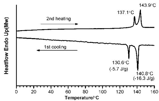
**ESI Fig. 38** DSC trace of compound **4j** run at 10 °C/min under N<sup>2</sup>.
