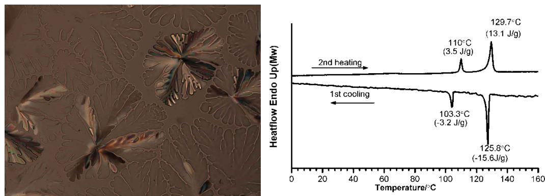
**ESI Fig. 39** Dendritic texture of compound **4k** sandwiched between clean glass slides on cooling from isotropic phase at 125 °C (left), this texture which indicated a Col<sub>h</sub> phase was observed by POM with 45° angle and did not show any changes when cooled to room temperature; DSC trace of compound **4k** run at 10 °C/min under N<sup>2</sup> (right).
