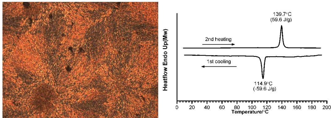
**ESI Fig. 28** Crystalline texture observed by POM with 90° angle of compound **4c** sandwiched between clean glass slides on cooling from isotropic phase at 127 °C (left); DSC trace of compound **4c** run at 10 °C/min under N<sup>2</sup> (right).
