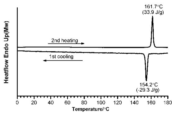
ESI Fig. 34 DSC trace of compound **4h** run at 10 °C/min under N<sup>2</sup>.
