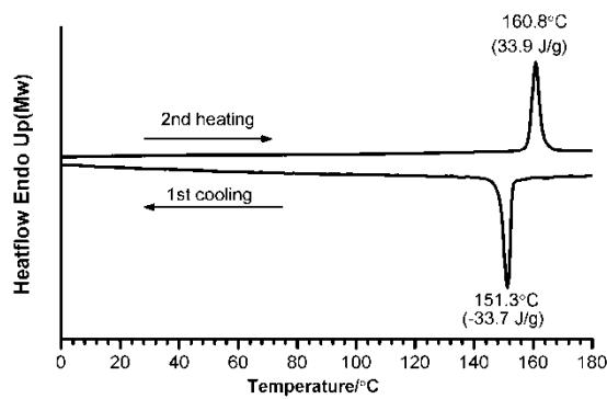
ESI Fig. 33 DSC trace of compound **4g** run at 10 °C/min under N<sup>2</sup>.
