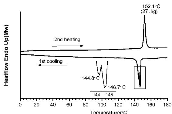
**ESI Fig. 36** DSC trace of compound **4i** run at 10 °C/min under N<sup>2</sup>.
