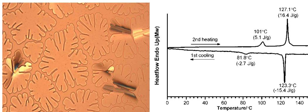
**ESI Fig. 31** Dendritic texture of compound **4e** sandwiched between clean glass slides on cooling from isotropic phase at 120 °C (left), this texture which indicated a Col<sub>h</sub> phase was observed by POM with 45° angle and did not show any changes when cooled to room temperature; DSC trace of compound **4e** run at 10 °C/min under N<sup>2</sup> (right).
