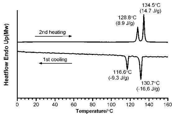
ESI Fig. 32 DSC trace of compound **4f** run at 10 °C/min under N<sup>2</sup>.
