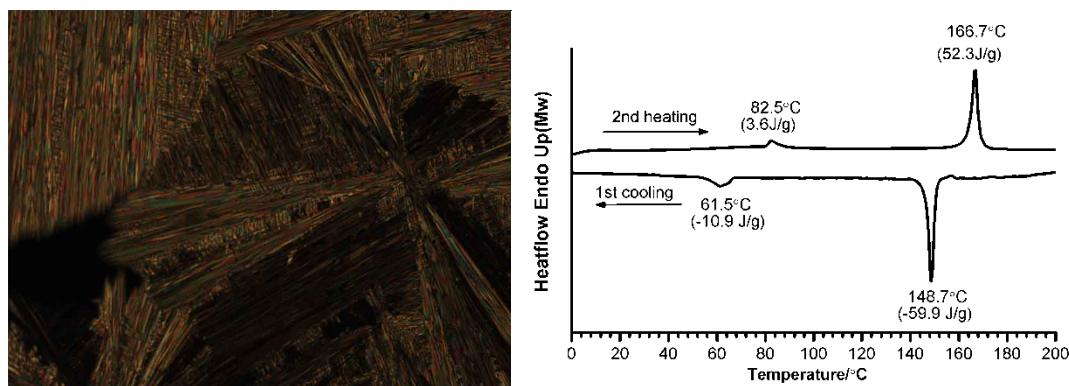
**ESI Fig. 26** Crystalline texture observed by POM with 90° angle of compound **4a** sandwiched between clean glass slides on cooling from isotropic phase at 140 °C (left); DSC trace of compound **4a** run at 10 °C/min under N<sup>2</sup> (right).
