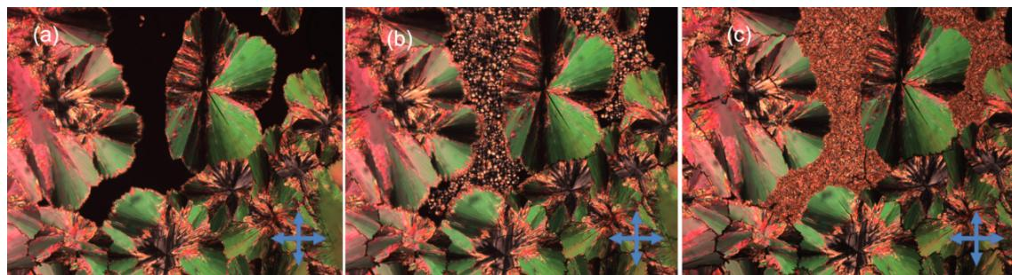
**ESI Fig. 29** texture of compound **4d** observed by POM when cooling from isotropic phase at (a) 85°C, (b) 75°C and (c) 70°C
