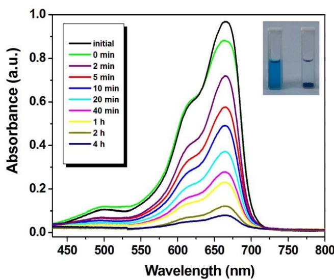
**Fig. S5** UV-vis spectra of the original and Zn(II)-MOF treated (30 mg) organic dye MB ( $5.0 \times 10^{-5}$  M) solution for various times. The insets are photos before and after the adsorption experiments under sunlight.
