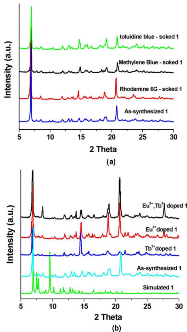
**Fig. S3** Powder XRD patterns for simulated, as-synthesized, lanthanide cations-doped Zn(II)-MOF and dye-soaked Zn(II)-MOF.
