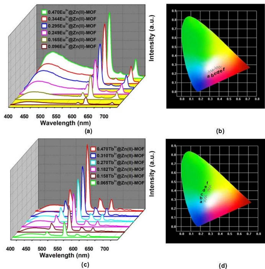
**Fig. S9** (a) Emission spectra of  $x\text{Eu}^{3+}$ @Zn(II)-MOF excitation at 359 nm. (b) CIE chromaticity coordinates and optical photographs of  $x\text{Eu}^{3+}$ @Zn(II)-MOF. (c) Emission spectra of  $x\text{Tb}^{3+}$ @Zn(II)-MOF excitation at 359 nm. (d) CIE chromaticity coordinates and optical photographs of  $x\text{Tb}^{3+}$ @Zn(II)-MOF.
