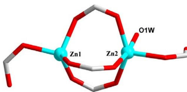
**Fig. S2** The “paddle-wheel” secondary building unit (SBU).
