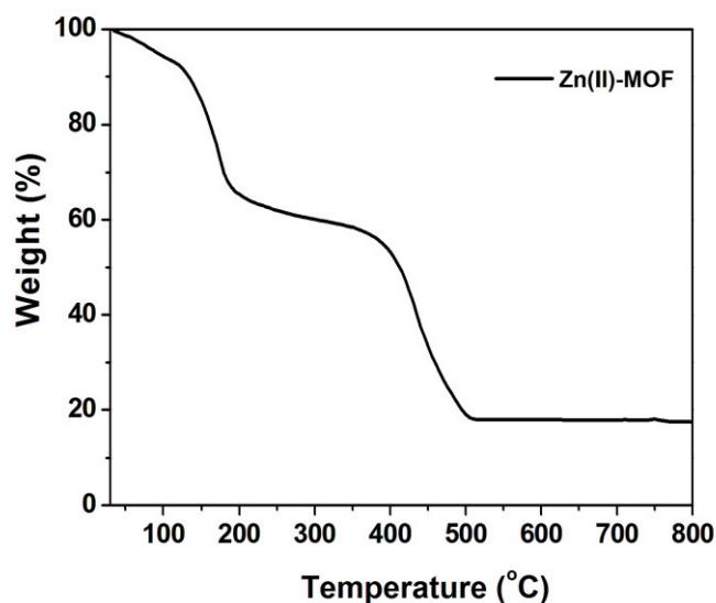
**Fig. S4** The thermogravimetric (TG) analysis curve of Zn(II)-MOF.
