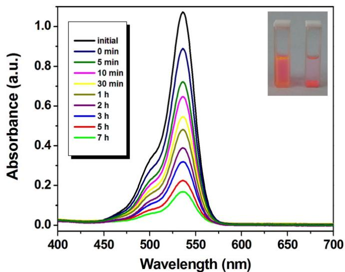
**Fig. S6** UV–vis spectra of the original and Zn(II)-MOF treated (30 mg) organic dye R6G ( $5.0 \times 10^{-5}$  M) solution for various times. The insets are photos before and after the adsorption experiments under sunlight.
