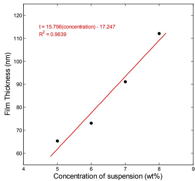
**Figure S3.** Effect of nanoparticle concentration on the thickness of discoidal TiO<sub>2</sub> nanoparticle films
