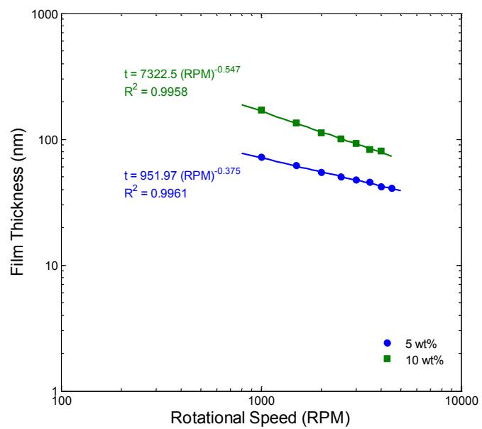
**Figure S1.** Effect of the rotational speed of spin coating on the thickness of spherical  $\text{TiO}_2$  nanoparticle films on glass slides.
