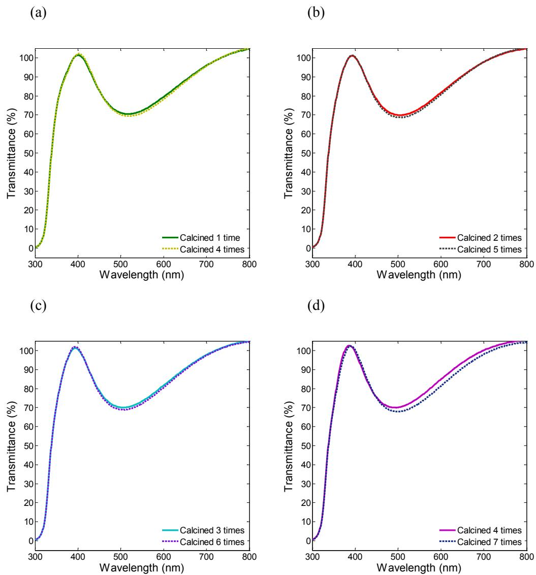
**Figure S4.** Effect of the total number of calcination processes on the transmittance spectra of 3-layer Bragg stacks on glass slides measured at normal incidence.
