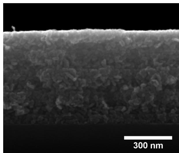
**Figure S5.** Cross sectional scanning electron microscopy (SEM) image of a 9-layer all-TiO<sub>2</sub> BS manufactured using the blocking-layer assisted spin coating method.
