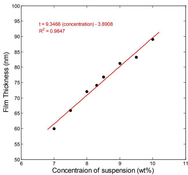
**Figure S2.** Effect of nanoparticle concentration on the thickness of spherical TiO<sub>2</sub> nanoparticle films
