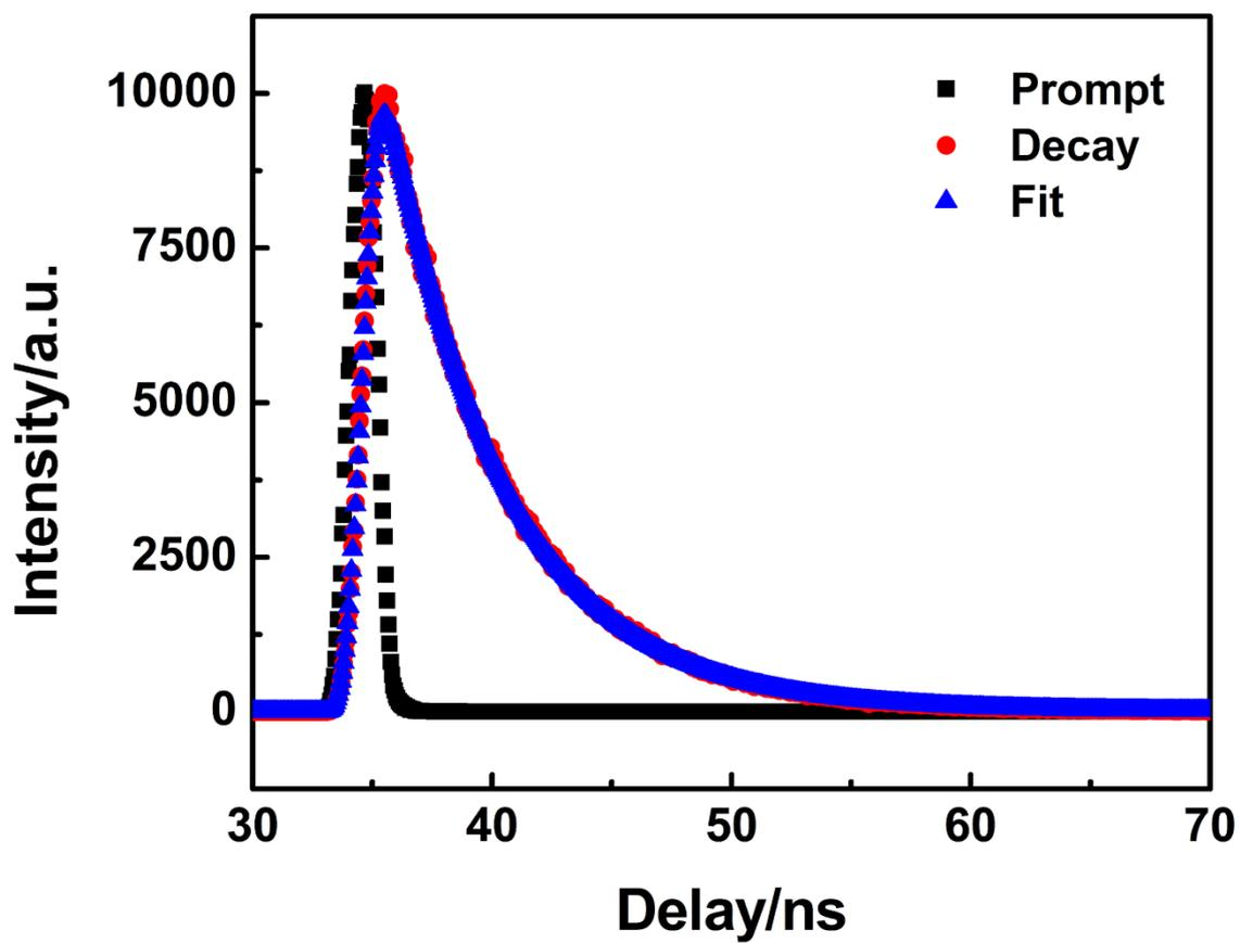
Figure S8. Time-resolved fluorescence decay of the *m*-CDs.
