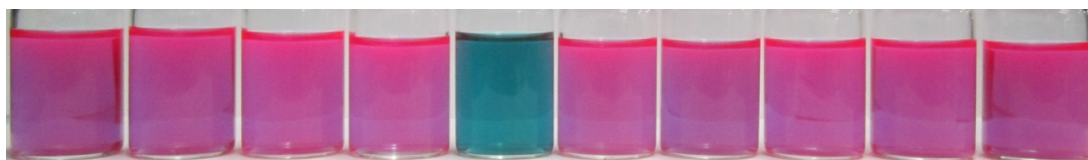
Figure S17: Color change induced upon addition of various (excess equivalents of perchlorate salts) metal ions to BODIPY 1 ( 5 \times 10^{-6} M) in \text{CH}_3\text{CN}/\text{PBS} (7:3; v/v, pH 7.4) under daylight: From left to right: (1) no metal ion, (2) \text{Na}^+ , (3) \text{K}^+ , (4) \text{Mn}^{2+} , (5) \text{Hg}^{2+} , (6) \text{Fe}^{2+} , (7) \text{Co}^{2+} , (8) \text{Ni}^{2+} , (9) \text{Cu}^{2+} and (10) \text{Zn}^{2+} respectively.
