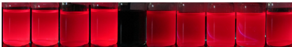
Figure S18: Color change induced upon addition of various (excess equivalents of perchlorate salts) metal ions to BODIPY 1 ( 5 \times 10^{-6} M) in \text{CH}_3\text{CN}/\text{PBS} (7:3; v/v, pH 7.4) under UV lamp: From left to right: (1) no metal ion, (2) \text{Na}^+ , (3) \text{K}^+ , (4) \text{Mn}^{2+} , (5) \text{Hg}^{2+} , (6) \text{Fe}^{2+} , (7) \text{Co}^{2+} , (8) \text{Ni}^{2+} , (9) \text{Cu}^{2+} and (10) \text{Zn}^{2+} respectively.
