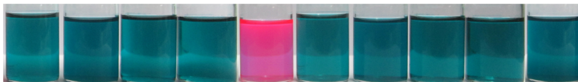
Figure S26: Color change induced upon addition of various (excess equivalents of \text{Bu}_4\text{N}^+ salts) anions to BODIPY 1 - \text{Hg}^{2+} complex ( 5 \times 10^{-6} M) in \text{CH}_3\text{CN}/\text{PBS} (7:3; v/v, pH 7.4) under daylight: From left to right: (1) \text{F}^- , (2) \text{CN}^- , (3) \text{N}_3^- , (4) \text{OH}^- , (5) \text{Cl}^- , (6) \text{Br}^- , (7) \text{I}^- , (8) \text{H}_2\text{PO}_4^- , (9) \text{HSO}_4^- and (10) \text{ClO}_4^- respectively.
