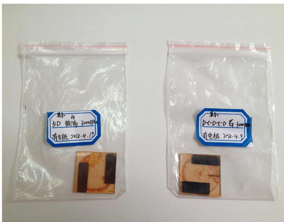
Figure S3. Samples after deposition of electrodes on a DAST film (Left), and a composite film (Right).
