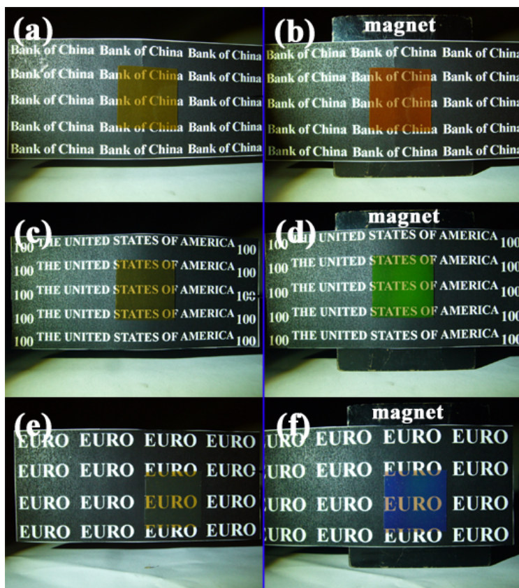
Figure S1. Digital photographs of the obtained double-layer flexible photonic display films containing carbon-capped superparamagnetic colloidal nanoparticles with different average particle size (a), (b) 190 nm, (c), (d) 135 nm and (e), (f) 115 nm.
