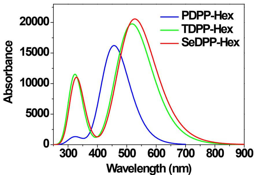
Figure S6. TD-DFT simulated absorption spectra of three DPP molecules.
