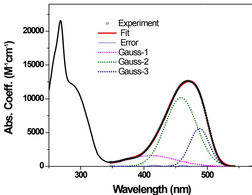
Figure S5. Absorption spectra overlapped with deconvoluted low energy band of PDPP-Hex.
