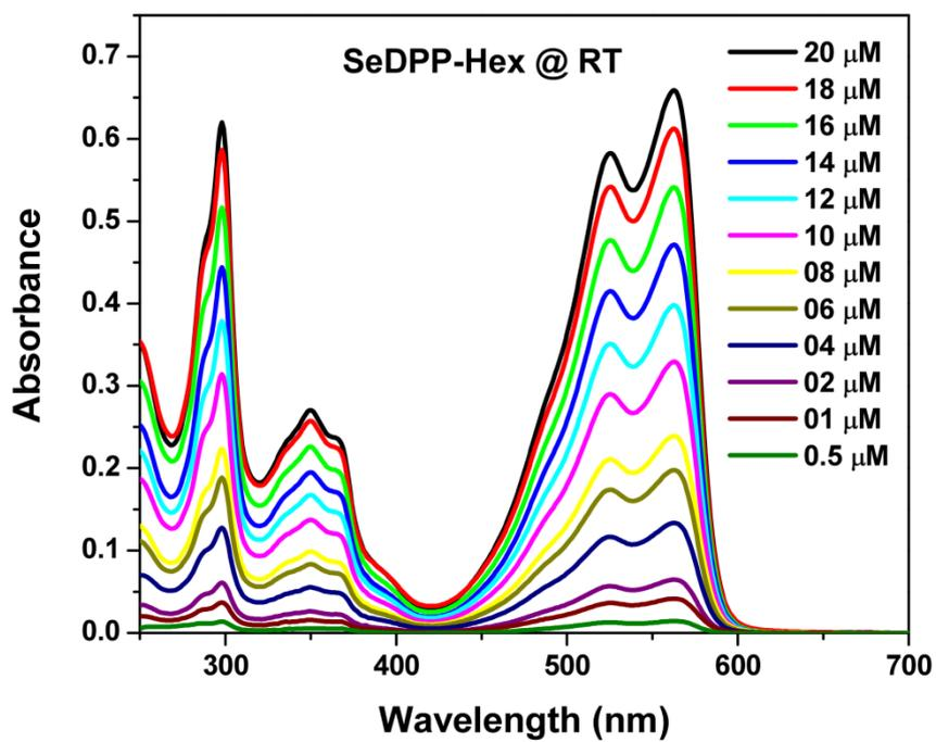
**Figure S7:** Room temperature concentration dependent absorption spectra of TDPP-Hex and SeDPP-Hex.
