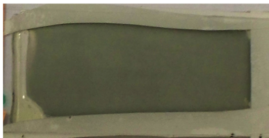
Fig. S2 a) Colored state and b) Bleached state for an electrochromic window with a 4cm 2 active area using the in situ procedure with 2.5 wt% ProDOT-Me 2 in the electrolyte gel.
