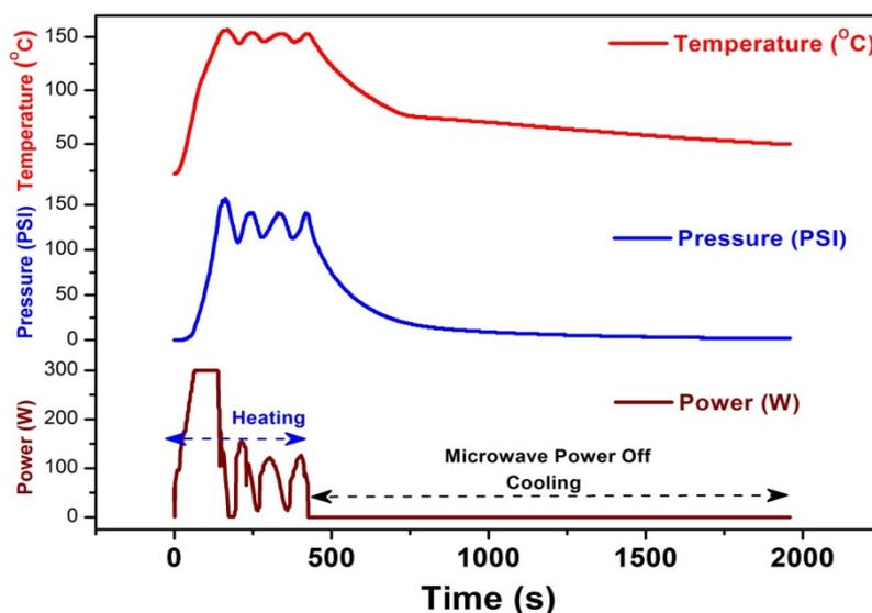
**Fig. S1** Variation of process parameters with time, during the microwave-assisted formation of GdOOH hierarchical structures.
