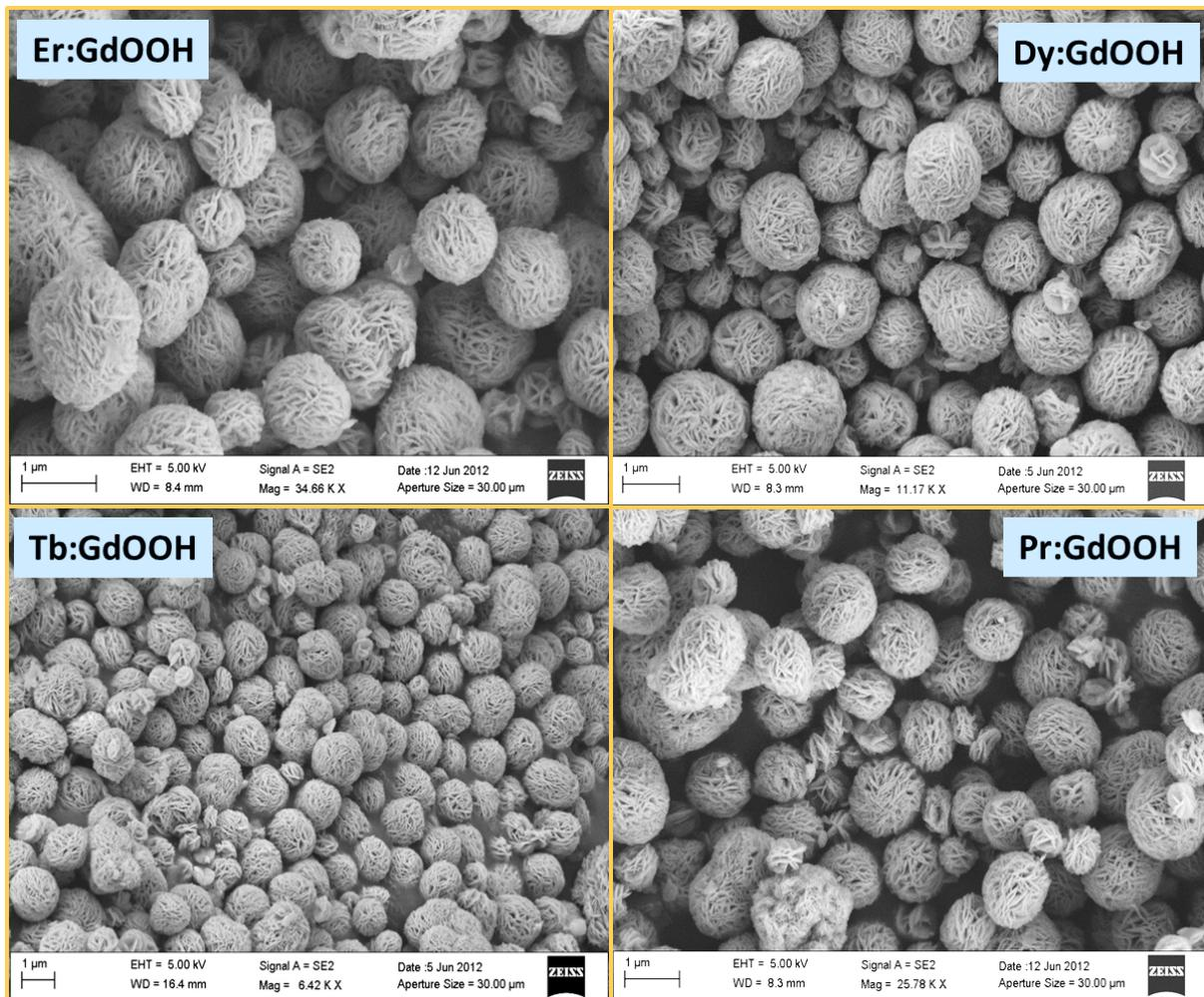
**Fig. S7** SEM micrographs of GdOOH spherical hierarchical structures prepared by the microwave irradiation route, and doped respectively with Er, Dy, Tb, and Pr,.
