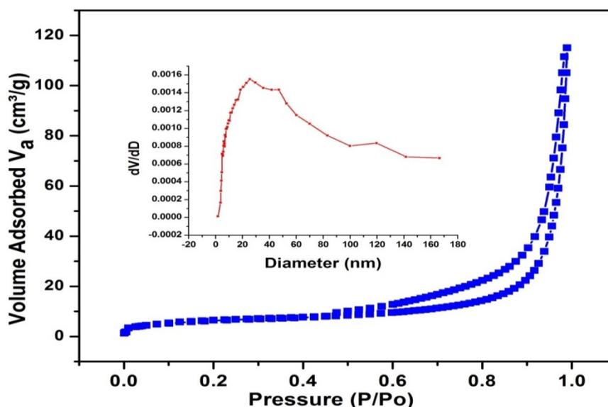
**Fig. S2** Adsorption and desorption isotherm for GdOOH microspheres. The inset shows BJH pore size distribution.
