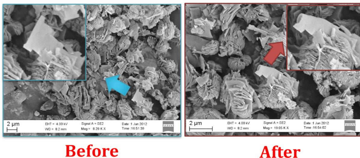
**Fig. S5** SEM micrographs of a single nanoflake before and after exposure to the e-beam.
