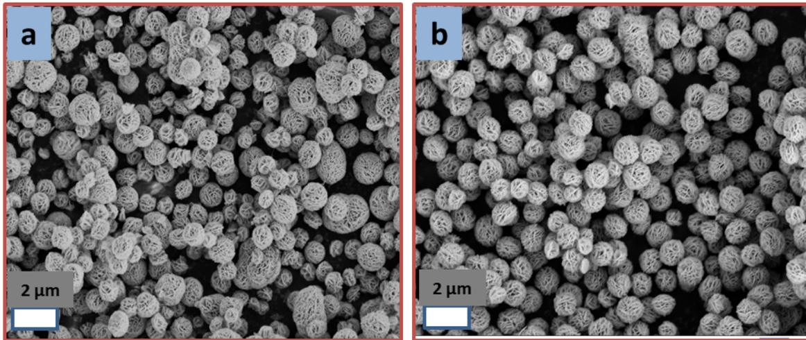
**Fig. S6** Morphology of the as-prepared GdOOH microspheres obtained (a) after run time of 8 min and (b) keeping the magnetic stirring on during microwave irradiation.
