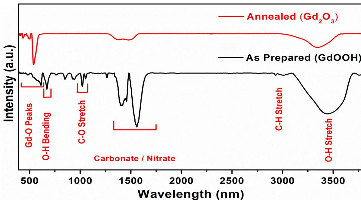
**Fig. S4** Infrared spectrum of as-prepared GdOOH product showing the presence of ethanolic peaks. No signature of ethanol is present in the annealed Gd<sub>2</sub>O<sub>3</sub> product as expected.
