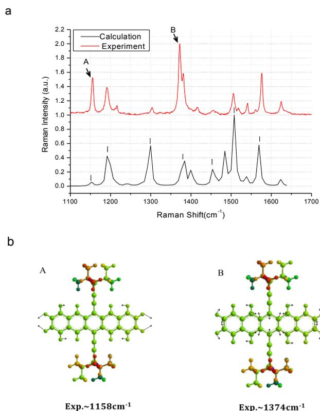
**Figure S1. (a) Comparison between the Raman spectrum of TIPS-Pentacene film (red), and calculated vibrational spectrum of gas-phase TIPS-Pentacene single molecule (black). The vibrational spectrum was calculated using Density Functional Theory at the B3LYP level of theory and a basis set of 6-31G\*. An empirical scaling factor of 0.9613 was applied to the calculated wavenumbers. (b) Selected C-H bending mode and aromatic C-C stretching modes of a TIPS-**
