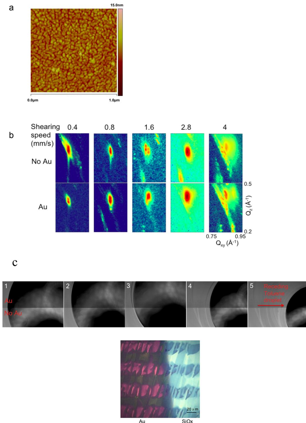
**Figure S6. a. AFM image of 9nm Au layer on the substrate.** This image shows that the gold covers the majority of the surface, and the surface roughness is around 0.796 nm, which demonstrate that the gold film is smooth. (As a reference, the surface roughness of a PTS modified Si wafer is  $\sim 0.5$  nm.<sup>2</sup>) **b. comparison of GIXD images of (101) peak of TIPS-pentacene sheared on substrates with 9nm Au layer vs.**
