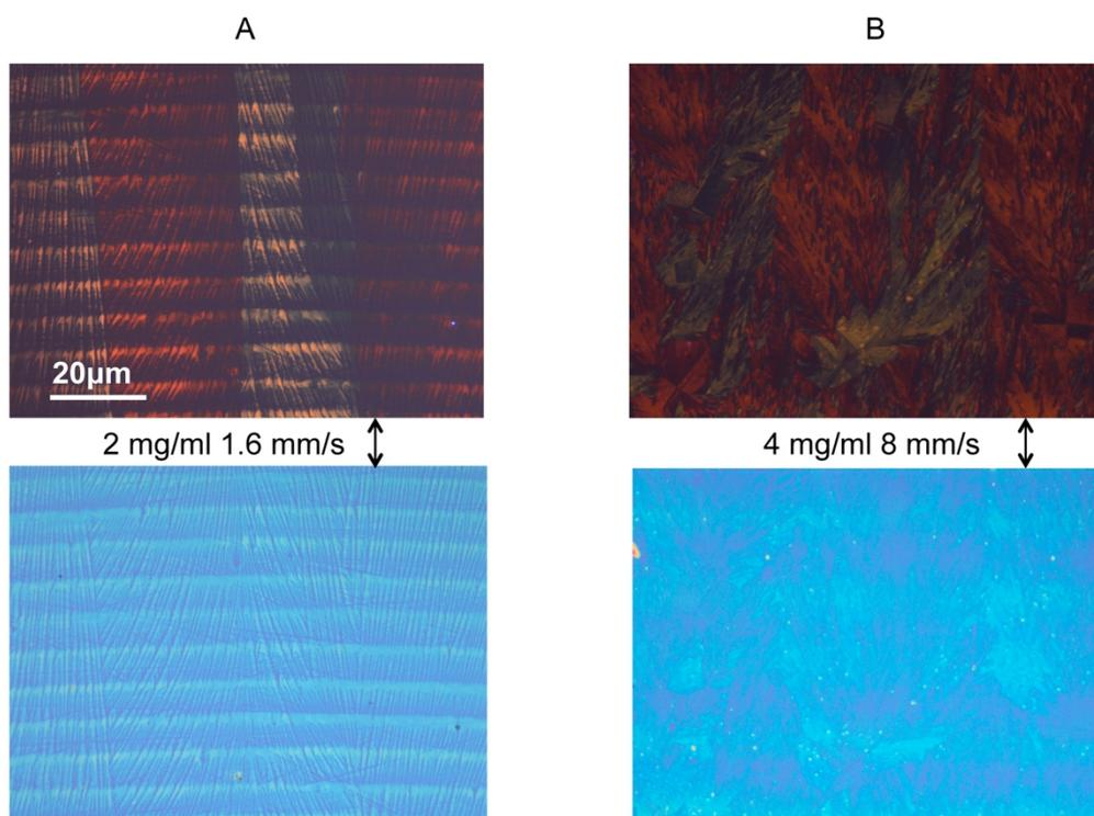
**Figure S9. Morphology comparison of TIPS-pentacene films with similar thickness prepared either with low concentration (A) or high shearing speed (B).** Upper images are taken under cross-polarized optical microscope. All images are of the same scale. These optical images show that the film prepared with low concentration and low speed has a better crystalline alignment.
