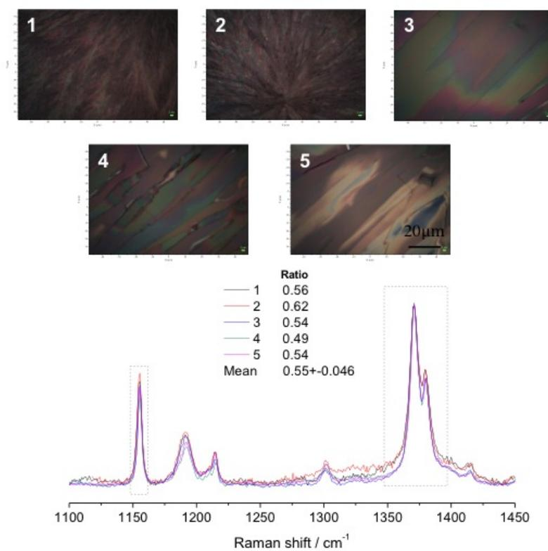
**Figure S4: Optical images and Raman spectra of TIPS-pentacene drop-casted films at different locations.**
