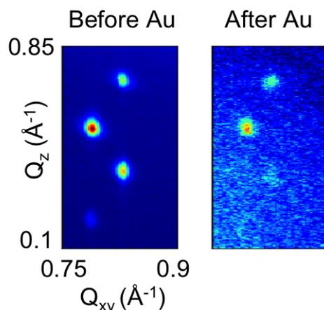
**Figure S7. GIXD images showing (010) and (101) peak positions before and after deposition of 9nm Au on the film top surface.** Thin films were prepared by shearing at 90°C from 2mg/ml toluene solution at 0.8mm/s. The GIXD was taken with sample in-plane rotation (phi scan). After depositing Au layer, the peak intensities decrease because of X-ray scattering from Au. The peak positions did not change after Au deposition, indicating that the molecular packing was not affected by Au deposition.
