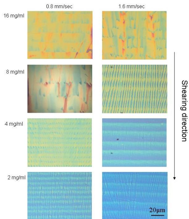
**Figure S3: Optical image of TIPS-pentacene films deposited from different concentration solutions.**
