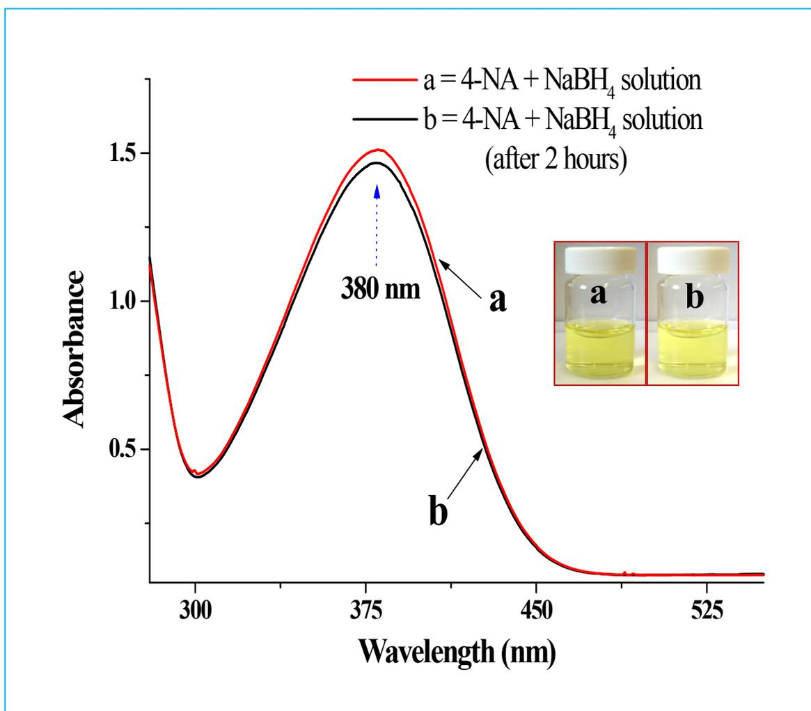
**Figure S-3.** The UV-Vis absorption spectrum of a mixture of 4-NA with  $\text{NaBH}_4$  just after mixing (curve a) and after aging the mixture for 2 hour (curve b). Inset shows the camera image of the two solutions.
