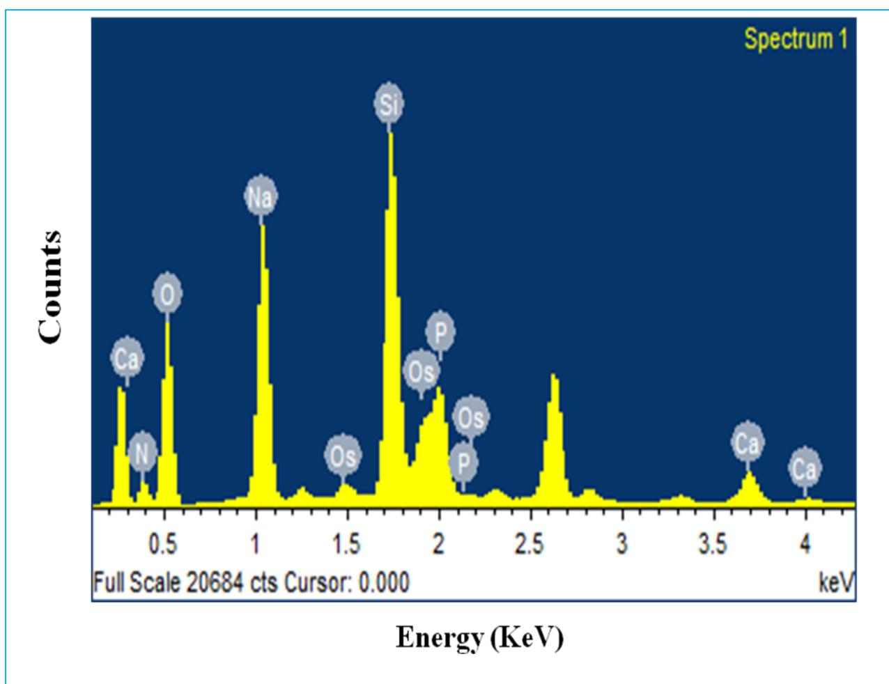
**Figure S-1:** The energy dispersive X-ray spectroscopic (EDS) analysis of the self-assembled Os NCs in DNA having different peaks of Os, O, N, P, Si and Ca.
