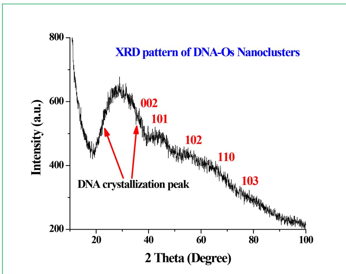
**Figure S-2.** The X-ray diffraction (XRD) pattern of the self-assembled Os NCs on DNA. The diffraction observed from the (002), (101), (102), (110) and (103) planes of hexagonally close pack (hcp) Os NCs.
