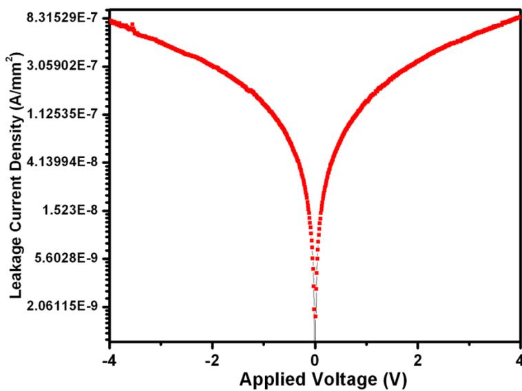
Figure S6. Leakage current density ( $\text{A}/\text{mm}^2$ ) measurement for the dehydrated sample **1'**.
