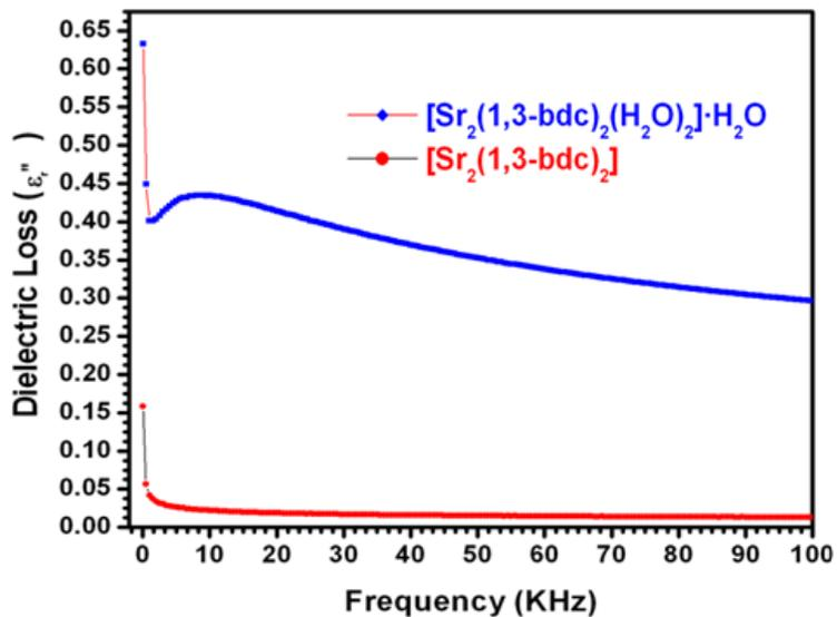
Figure S5. Dielectric loss vs frequency curves of pellet sample **1** and dehydrated compound **1'**.
