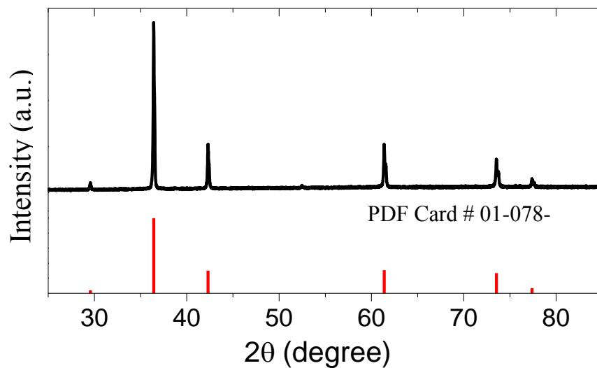
**Figure S1.** Powder X-ray diffraction pattern for the  $\text{Cu}_2\text{O}$  sample. The positions of XRD peaks match the  $\text{Cu}_2\text{O}$  peaks from the standard PDF card.
