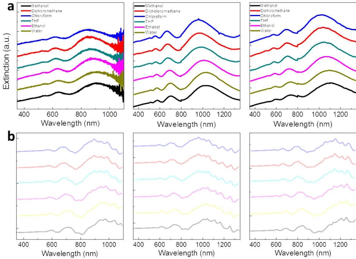
**Figure S4.** Extinction spectra of  $\text{Cu}_2\text{O}$  microcrystals with different morphologies suspended in different media, (a) from experimental, and (b) by calculation.
