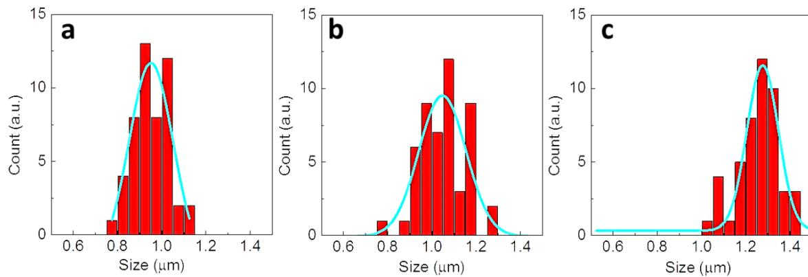
**Figure S2.** Size distributions of as synthesized  $\text{Cu}_2\text{O}$  microcrystals with precursors' formation under different temperature (a-c, 16°C, 10°C, and 5°C). The lengths of their edge are  $950 \pm 164$ ,  $1050 \pm 128$ , and  $1280 \pm 168$  nm, respectively. The approximated diameters in stimulation for those microcrystals are 1300, 1400, and 1700 nm, respectively.
