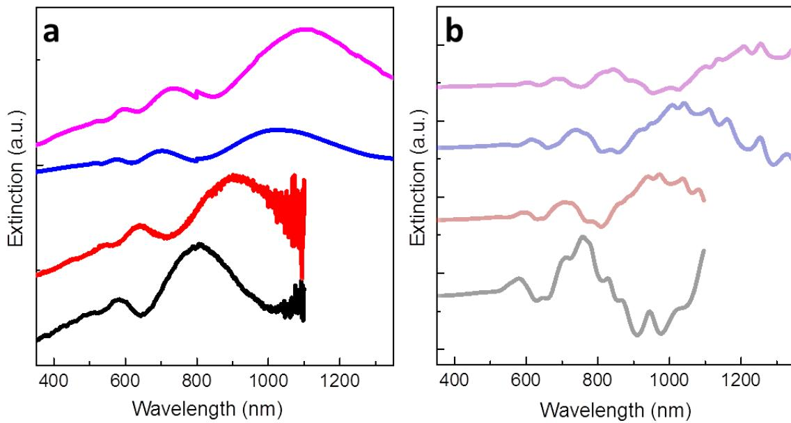
**Figure S3.** Experimental (a) and calculated (b) extinction spectra of  $\text{Cu}_2\text{O}$  microcrystals with precursors at different temperature suspended in methanol.
