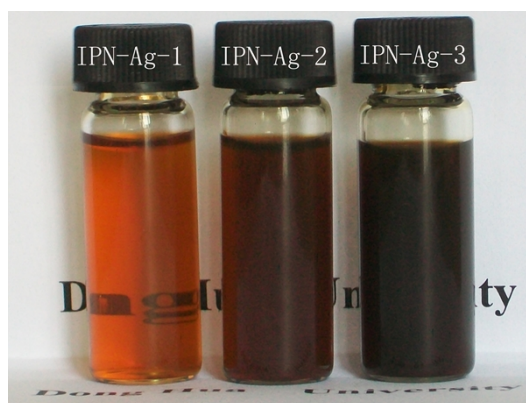
Figure S1 Appearance picture of AgNPs/(PNIPAM/PAA IPN) hybrid microgels aqueous dispersions with different AgNPs contents
