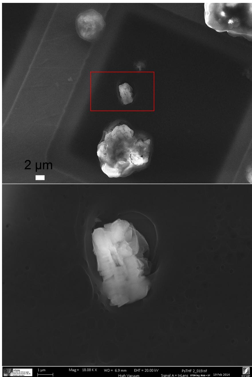
Figure S.4. SCO/PS hybrid material. Figure shows the 10  $\mu\text{m}$  cluster and below can be seen the morphological characteristics corresponding to SCO particle aggregates. Moreover the porous in the PS film are due to the THF.
