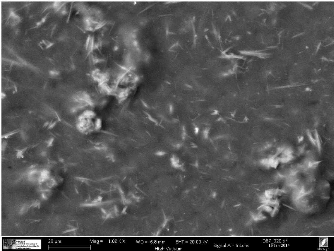
Figure S.12. Image at the top is an enlargement of the Figure 4.i for better visualization of the SCO particles forming fibers in D6. Fibers and larger clusters are observed.
