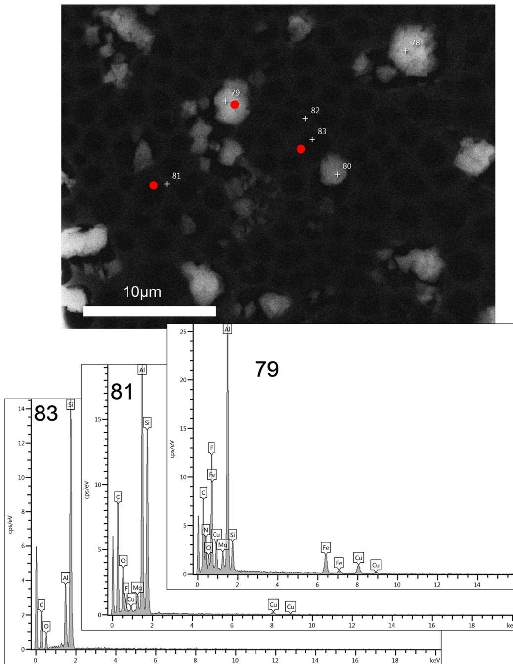
Figure S.7. Microelemental analysis for the SCO/PMMA in THF hybrid material in different localizations, (83): into the porous, (81): in the polymeric network and (79). The characteristics elements of the SCO material such as F, Fe and N are not observed neither in 83 nor 81.
