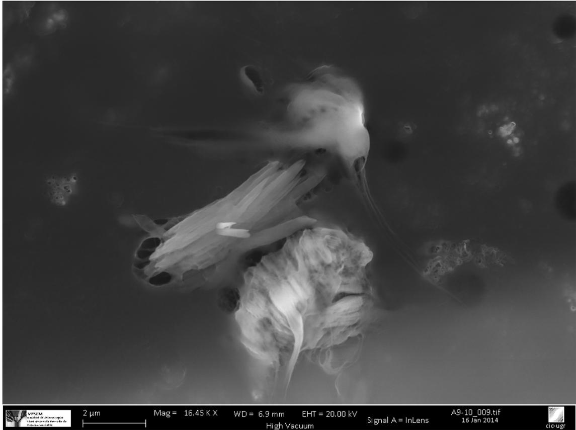
Figure S.11. Enlargement of the Figure 4.f for better visualization of the SCO particles in Nafion.
