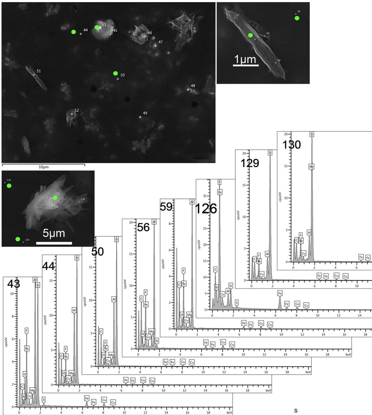
Figure S8. Microelemental analysis for the SCO/Nafion hybrid material. Located analysis points in the background (44, 50, 59, 129 and 130) reveal that iron, a common elements for the SCO material, is present involving a possible dissolution of the SCO particles and so, a subsequent morphology change to fibers like particles.
