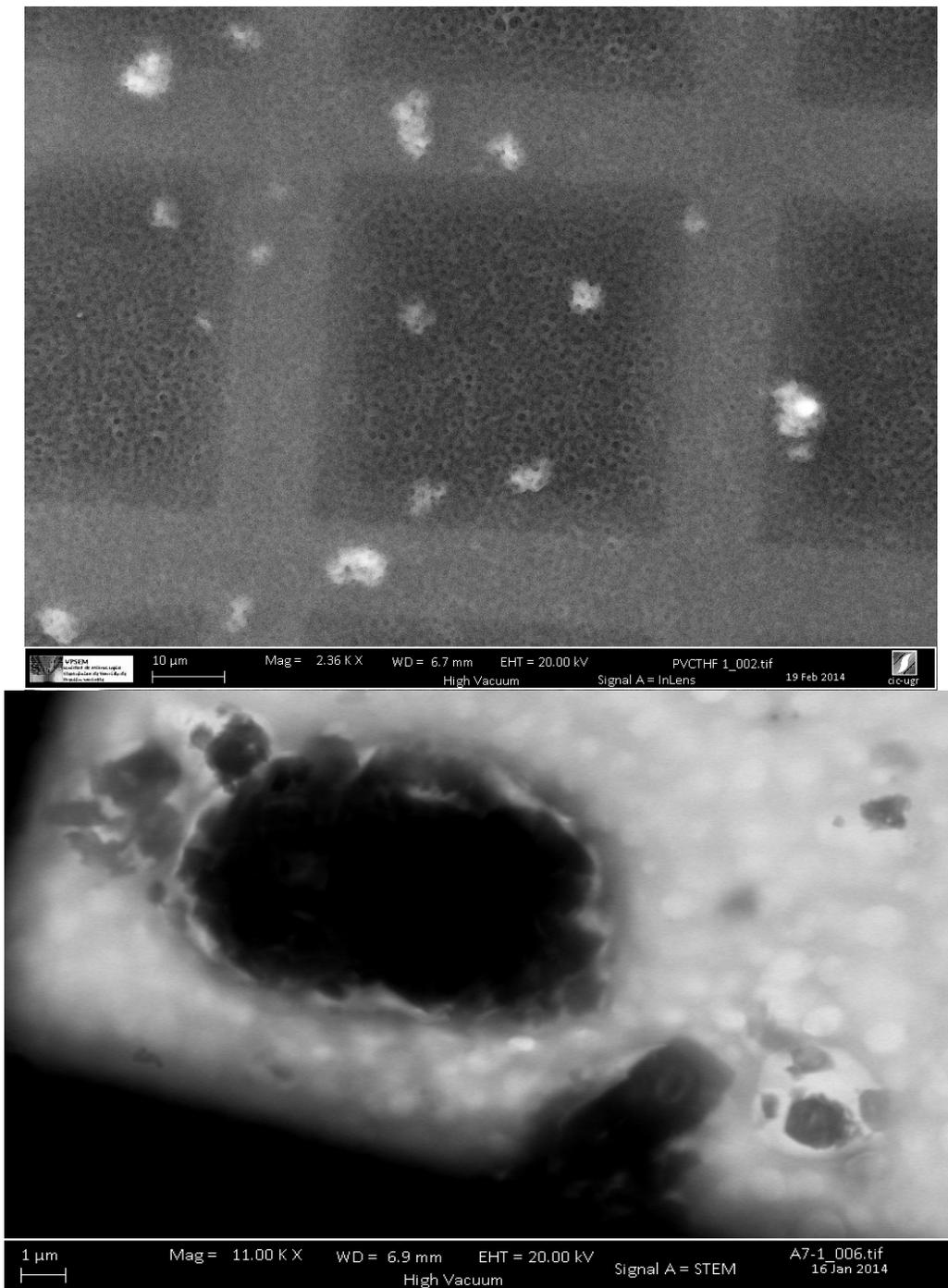
Figure S.2 is Figure S.2. SCO/PVC hybrid material. The cluster formation due to single SCO crystal aggregation when using PVC. Moreover the porosity in the polymeric films is due to the use of THF as solvent.
