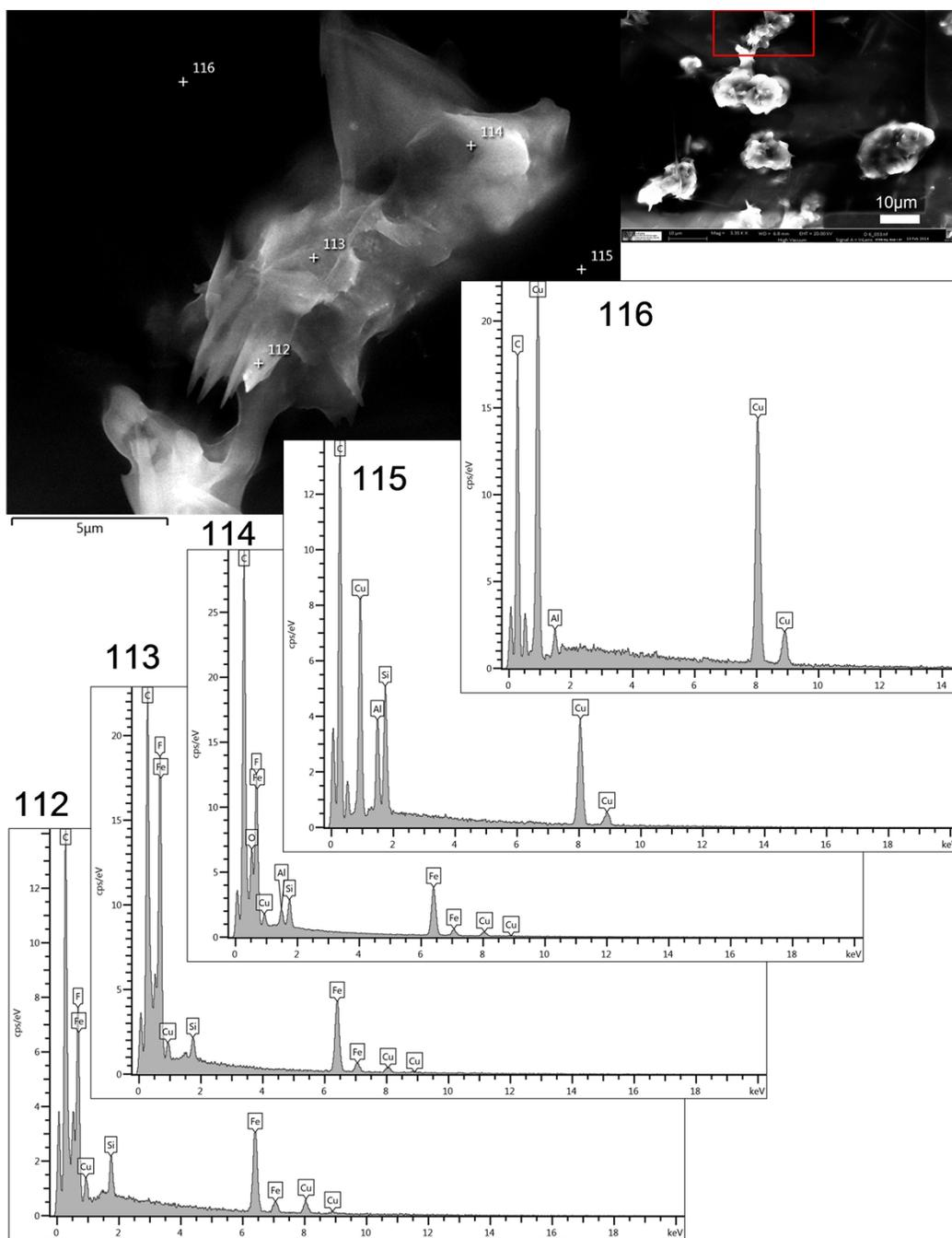
Figure S.9. Microelemental analysis for the SCO/D6 hybrid material. Inside the cluster (from 112 to 114 points) characteristics elements of the SCO material such as F and Fe are observed. Points 112 and 113 are located on the surface of around 8  $\mu\text{m}$  fiber. Points 115 and 116 correspond with the background. Top right shows clusters formation around 10-20  $\mu\text{m}$ . Large image is a red rectangle magnify.
