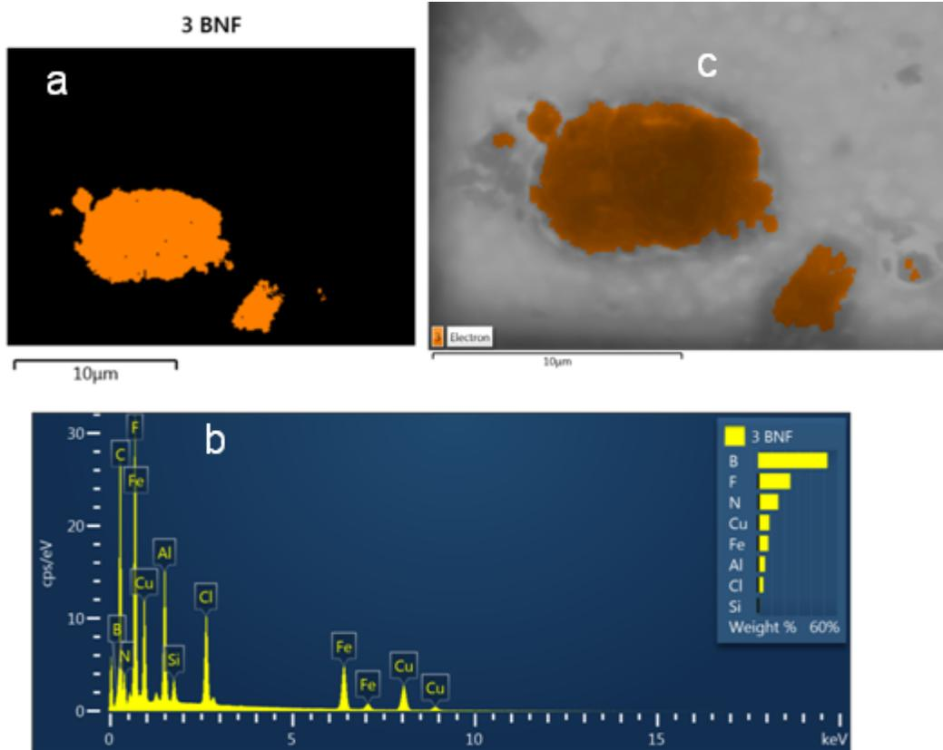
Figure S.3. Microelemental analysis for SCO/PVC hybrid material as extension of the analysis of the Figure 3.c and 3.d. It can be seen the elemental mapping for B, N and F and the correspondence with the STEM image.
