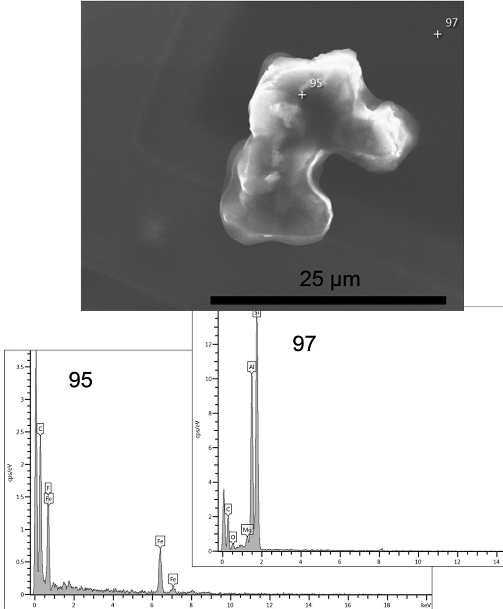
Figure S.5. Microelemental analysis for the SCO/PS hybrid material in the background (97) and on the material surface (95). The characteristics elements of the SCO material such as F and Fe are not observed in the background. The presence of C is assigned to the PS. On the other hand, mainly C and O were observed in the background which involves the SCO crystals are not affected by dissolution processes
