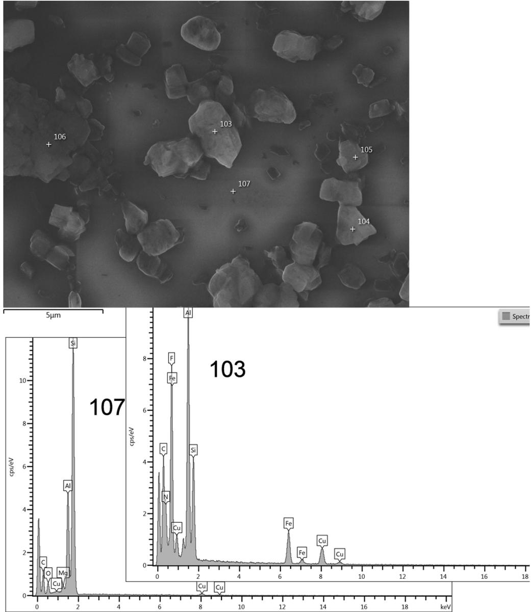
Figure S.6. Microelemental analysis for the SCO/PMMA in toluene hybrid material. In the background (107) and on the material surface (103). The characteristics elements of the SCO material such as F, Fe and N are not observed in the background (mainly C and O).
