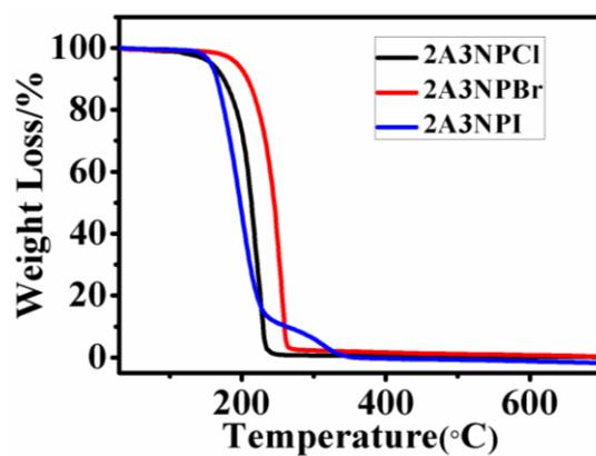
Figure S3. TGA curves of 2A3NPI, 2A3NPBr and 2A3NPI.
