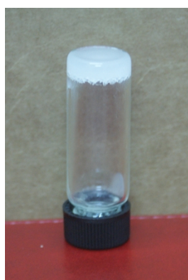
Figure S19 The photograph of IL-MOF-253-Ln after cooled completely in the room temperature.
