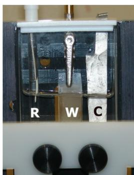
**Figure S5.** Setup of customized optical glass cell for Spectro-Electrochemical measurements. W: FTO glass/EFS Working Electrode; C: Platinum Plate Counter Electrode; R: aqueous Ag/AgCl Reference Electrode.
