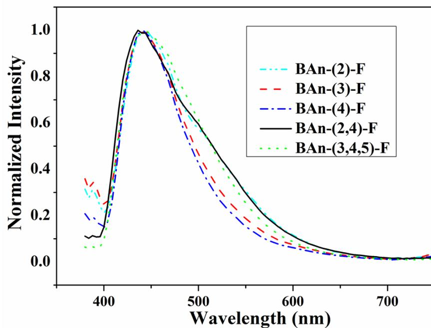
Fig. S3 EL spectrum of non-doped devices at  $10 \text{ mA cm}^{-2}$ .
