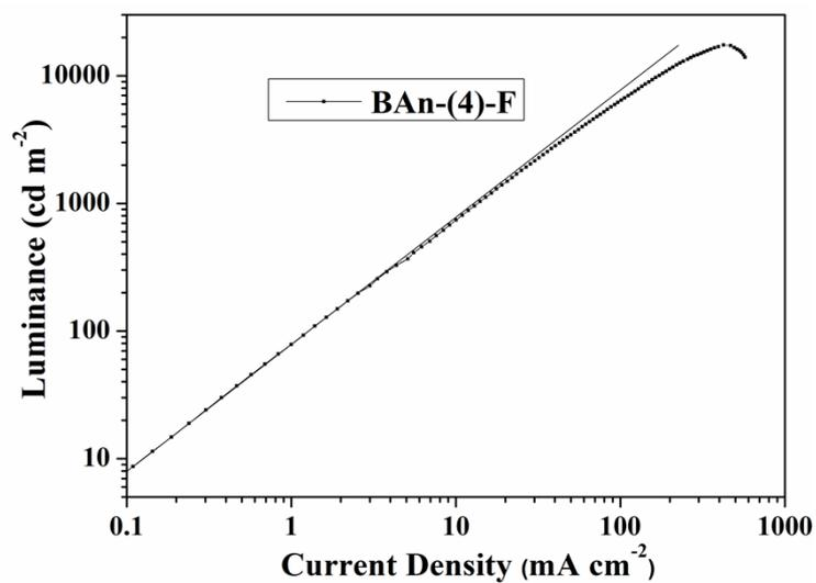
**Fig. S2** The current–brightness characteristic of the device based on the host BAn-(4)-F.
