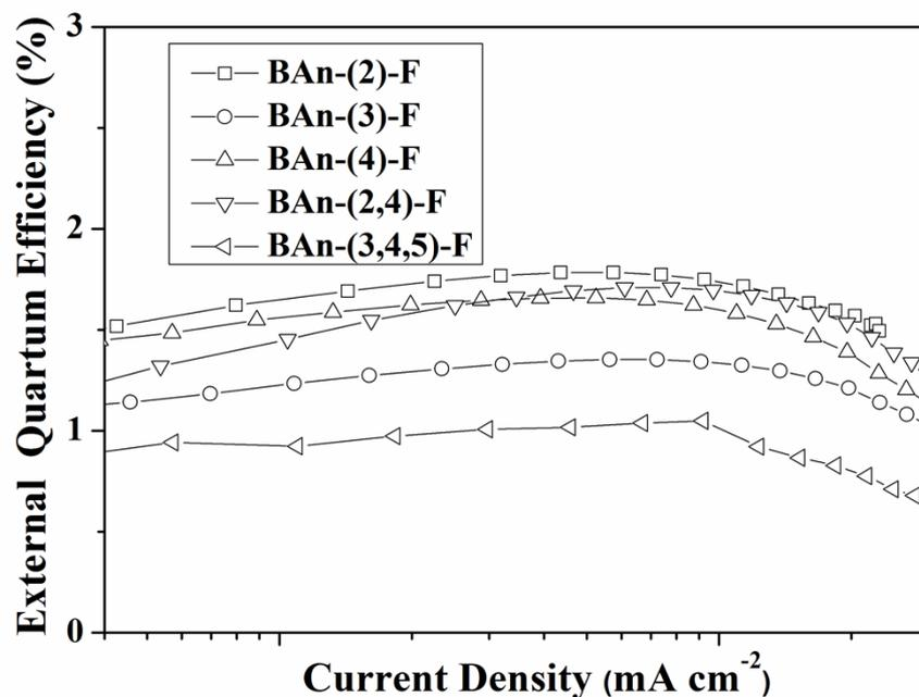
Fig. S5 External quantum efficiency (EQE) at different current densities for non-doped devices.
