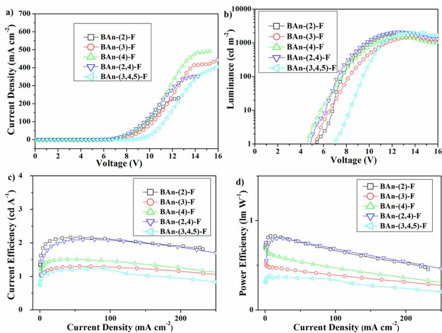
Fig. S4 a) Current density–voltage curves, b) Brightness–voltage curves, c) Current efficiency–current density curves, and d) Power efficiency–current density curves for the devices employing BAnFs as a non-doped emitter.
