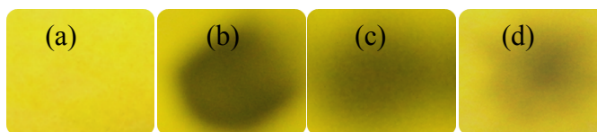
Fig. S43 Photographs (under 365 nm UV light) of fluorescence quenching of nanoaggregates of derivative 9 on test strips for the visual detection of small amount of PA (A) test strip; PA of different concentration (b) 10^{-4} M (c) 10^{-6} M (d) 10^{-8} M.
