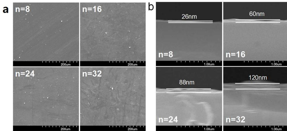
**Fig. S6** The top (a) and side (b) view SEM profiles of the  $(\text{Tb}(\text{acac})_3\text{Tiron/LDH})_n$
