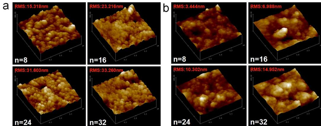
**Fig. S7** AFM images of the  $(\text{LC/LDH})_n$  TFs for a)  $(\text{Eu}(\text{DBM})_3\text{bath/LDH})_n$  ( $n=8-32$ ) TFs; b)  $(\text{Tb}(\text{acac})_3\text{Tiron/LDH})_n$  ( $n=8-32$ ) TFs. Their RMS surface roughness values are also supplied.
