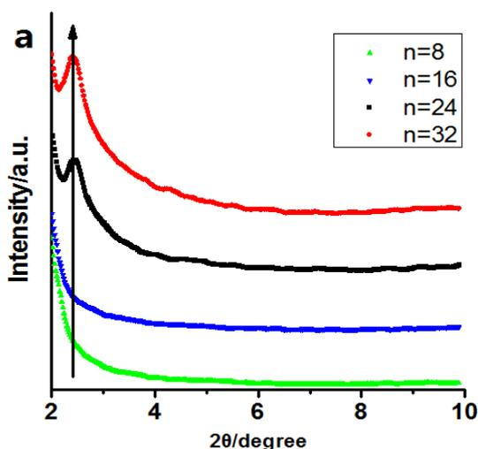
**Fig. S4** The XRD profiles for  $(LC/LDH)_n$  TFs. a)  $(Eu(DBM)_3bath/LDH)_n$  ( $n=8-32$ ) TFs; b)  $(Tb(acac)_3Tiron/LDH)_n$  ( $n=8-32$ ) TFs.
