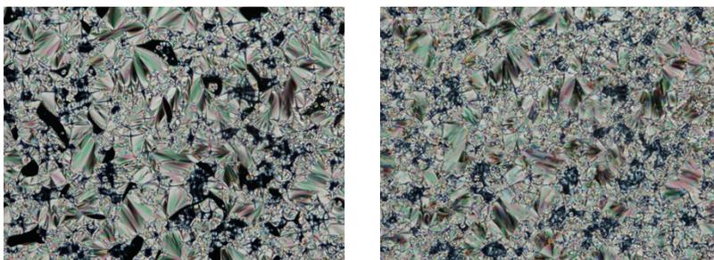
**Fig. S2.** Polarized photomicrographs of compound **QL18-3** at 72 °C in the SmA phase (left) and at 64 °C in the SmC phase (right).
