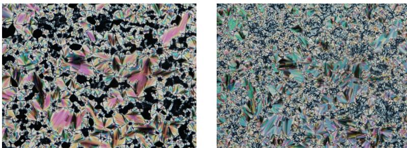
**Fig. S1.** Polarized photomicrographs of compound **QL13-3** at 65 °C in the SmA phase (left) and at 58 °C in the SmC phase (right).
