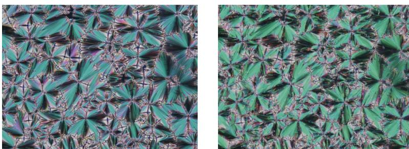
**Fig. S6.** Polarized photomicrographs of compound **QL19-6** as an unaligned 10  $\mu\text{m}$  film at  $T-T_{AC} = +1\text{K}$  (left) and at  $T-T_{AC} = -15\text{ K}$  (right).
