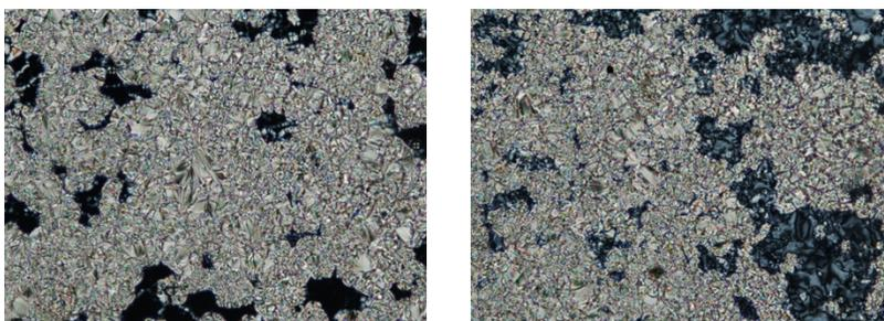
**Fig. S3.** Polarized photomicrographs of compound **QL19-6** at 75 °C in the SmA phase (left) and at 60 °C in the SmC phase (right).
