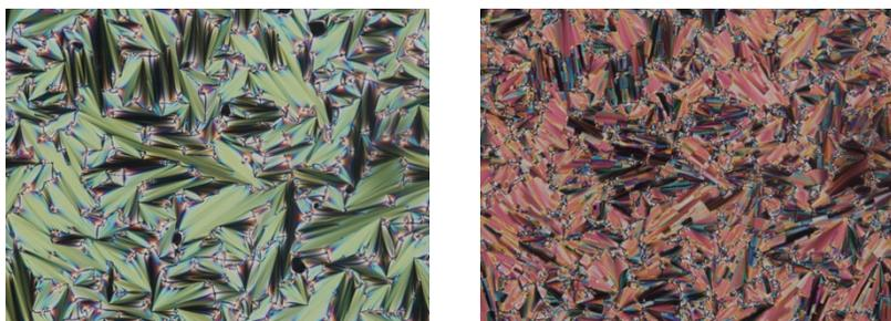
**Fig. S4.** Polarized photomicrographs of compound **QL13-3** as an unaligned 10  $\mu\text{m}$  film at  $T - T_{AC} = +1\text{K}$  (left) and at  $T - T_{AC} = -15\text{K}$  (right).
