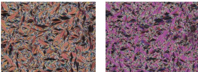
**Fig. S5.** Polarized photomicrographs of compound **QL18-3** as an unaligned 10  $\mu\text{m}$  film at  $T-T_{AC} = +1\text{K}$  (left) and at  $T-T_{AC} = -15\text{ K}$  (right).
