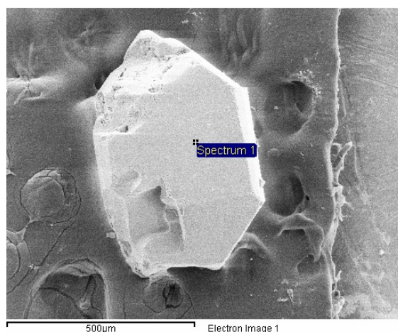
Figure S4. Morphology of a \text{SrCu}(\text{OH})_3\text{Cl} crystal under scanning electron microscope. Marked spot denotes the position where the EXD spectrum in Figure S3 was measured.
