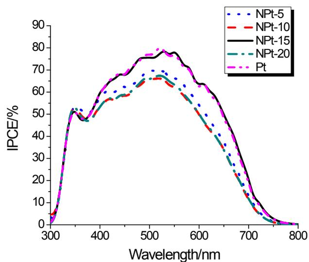
Fig. S1 Photocurrent action spectra of the DSSCs with NPs and Pt counter electrode.
