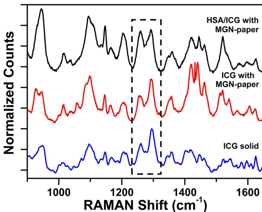
**Figure S1.** SERS detection of 42  $\mu\text{M}$ :21  $\mu\text{M}$  HSA:ICG with MGN-paper dipstick (black). SERS detection of 20  $\mu\text{M}$  ICG with MGN-paper dipstick (red). Raman of solid ICG (blue). Spectra were normalized to their respective 1294  $\text{cm}^{-1}$  peaks and then stacked for comparison. Boxed region focuses on the intensity ratios of the 1258:1294  $\text{cm}^{-1}$  peaks for each sample.
