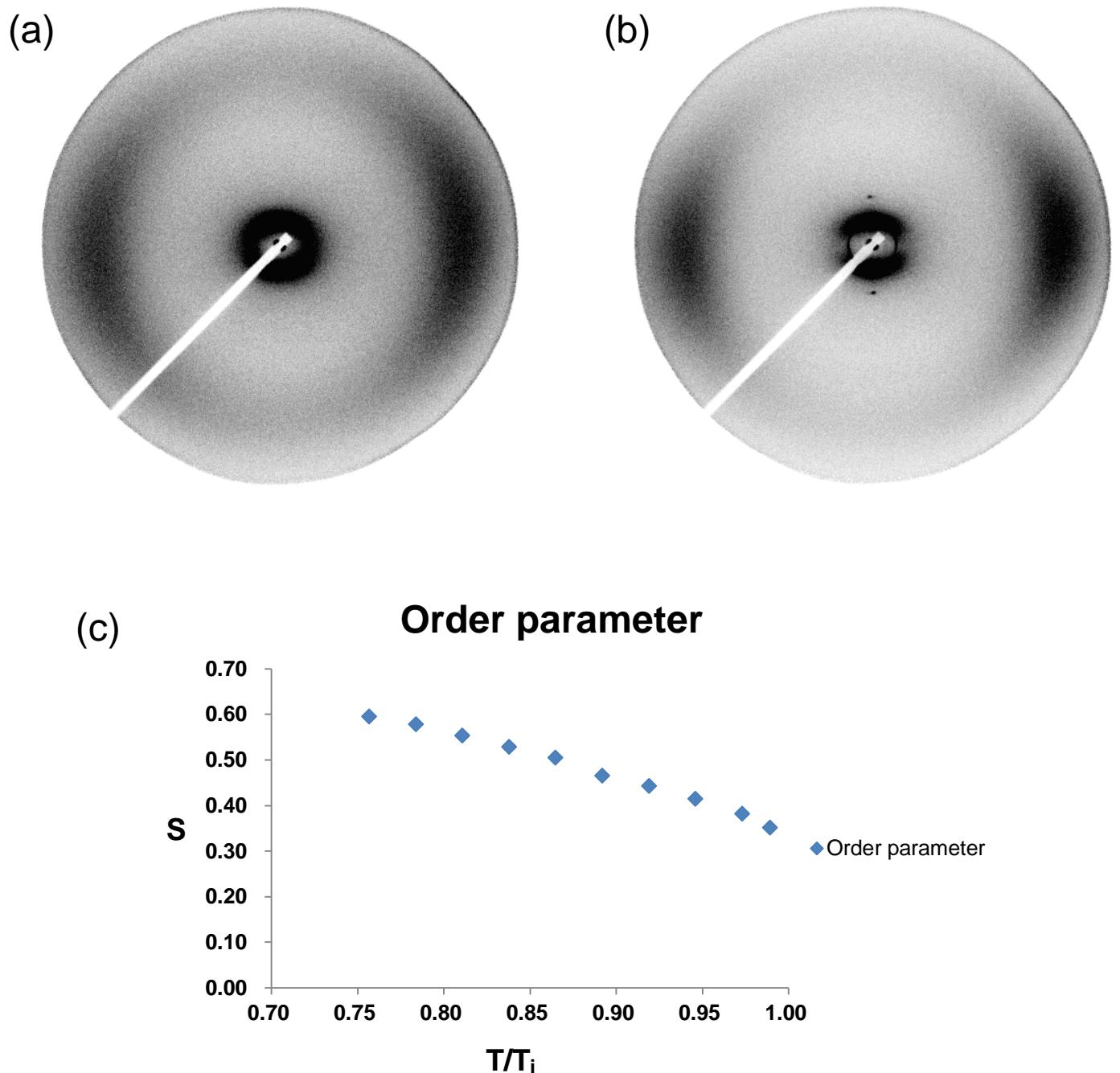
Figure S1. 2D Oriented WAXD patterns at (a) nematic phase ( $175\text{ }^\circ\text{C}$ ) and (b) smectic phase ( $140\text{ }^\circ\text{C}$ ). © Temperature dependence of order parameters calculated from the WAXD investigation.  $T_i$  indicates Isotropic–nematic transition temperature upon cooling process.
