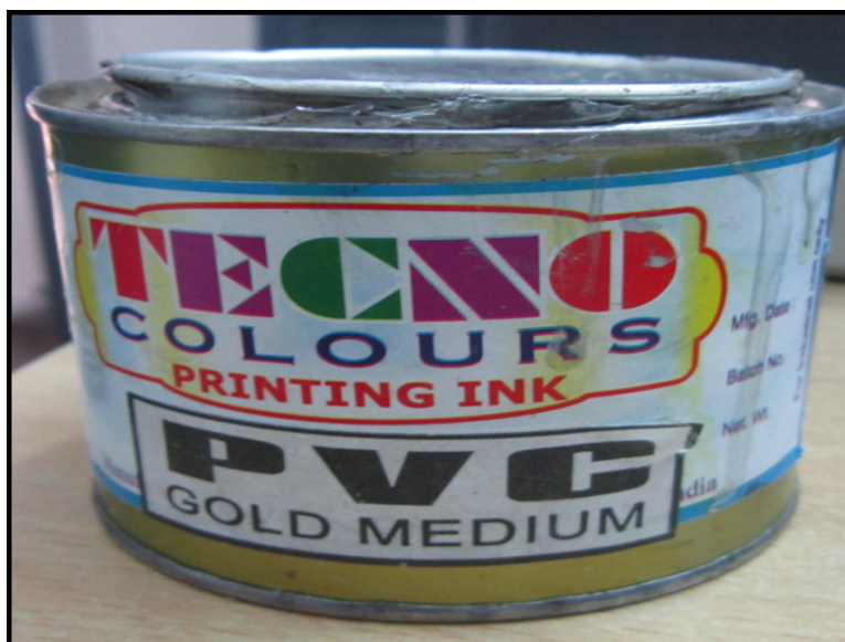
Fig. S1 Commercially available PVC gold medium used for ink preparation. The use of PVC gold medium is well known for screen printing which is major advantage in present case to choose PVC gold medium.
