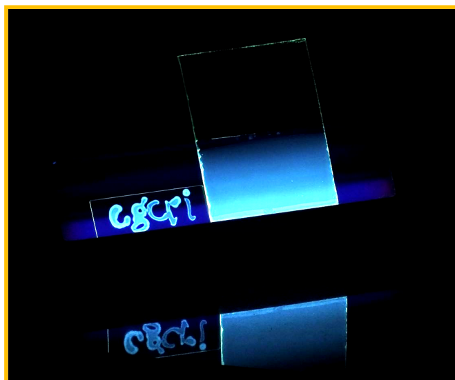
Fig. S1 Digital picture of CNDs–ORMOSIL used for writing on a glass slide and scratch resistant film on a 6 x 6 inch 2 glass under UV-lamp of wavelength 365 nm. Bottom is the reflection image.
