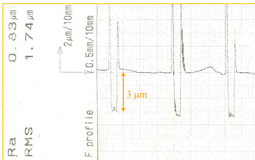
Fig. S2 Profilometric traces at 3 different places of one representative CND-ORMOSIL film deposited on glass substrate. Surface of the as-prepared film (dried at room temperature) was first scratched with a sharp steel blade followed by heat treatment at 70 °C for 6 h.
