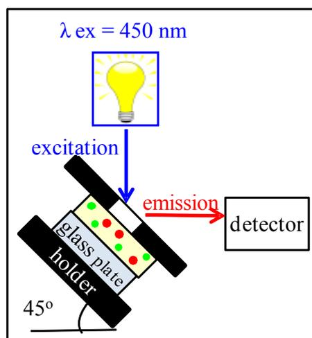
Figure S1. Schematic illustrations of: (a) experimental setup used to measure emission spectra of QDPLC films, and (b) interaction between emission light (including both extraction light and guiding light) and QD.
