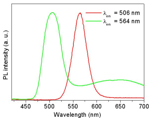
Figure S2. PL spectra of as-prepared CdSe core NCs dispersed in toluene.
