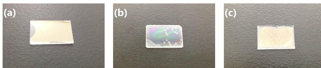
Fig. S5 Photographs of ~100 nm thin films deposited on quartz substrates after one week. (a) Vacuum-deposited CBP film; (b) spin-coated CBP film annealed at 50 °C for 10 min; (c) spin-coated CPCB film annealed at 220 °C for 10 min. The spin-coated CBP film partly crystallized, while the vacuum-deposited CBP and spin-coated CPCB films were still amorphous.
