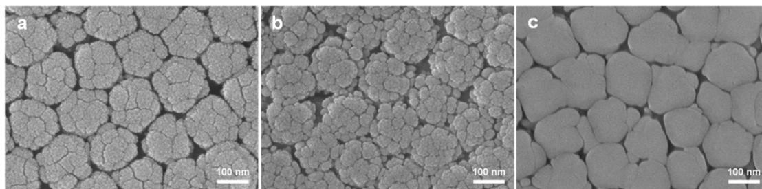
**Figure S1** FE-SEM images of Ag SERS substrates after deposition of Ag nanoparticles onto the SiO<sub>2</sub> colloidal crystal template for (a) 90 s, (b) 180 s, and (c) 300 s, respectively.
