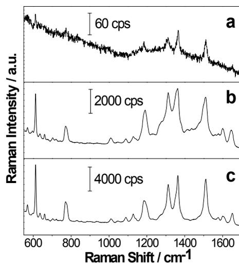
**Figure S2** (a) Normal Raman spectrum of  $10^{-2}$  M R6G solution. Laser power: 80 mW. SERS spectrum of  $10^{-4}$  M R6G solution acquired from SiO<sub>2</sub> colloidal crystal-assisted (b) Au and (c) Ag SERS substrates (the deposition time were both 180 s), respectively. Laser power: 0.8 mW.
