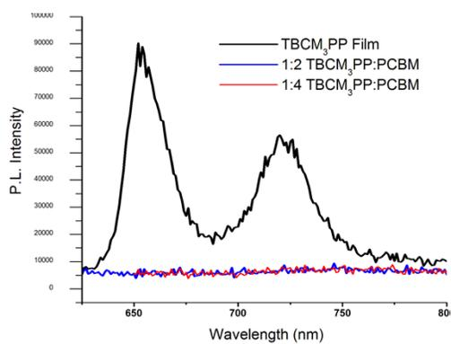
**Figure S4.** Steady-state PL quenching of TBCM<sub>3</sub>PP thin films with 1:2 and 1:4 PCBM by weight.
