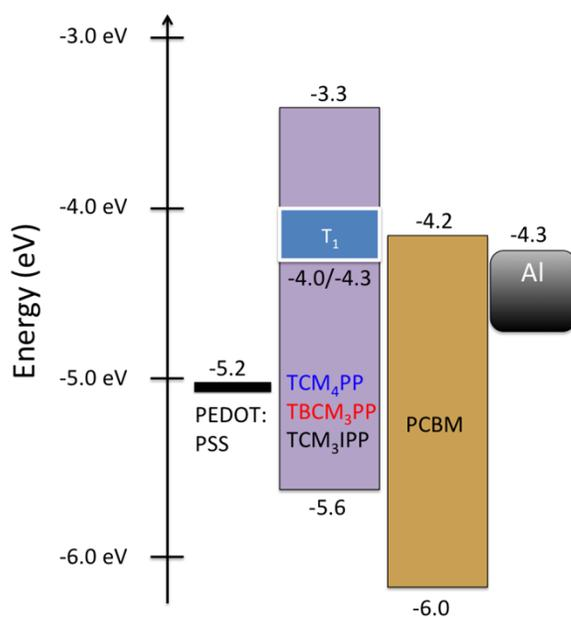
**Figure S6.** Energy level diagram of porphyrin (TCMPP derivatives) - PCBM organic photovoltaic devices with approximate porphyrin triplet state  $T_1$  energies.
