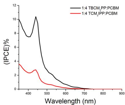
**Figure S3.** IPCE % spectrum of TBCM<sub>3</sub>PP:PCBM and TCM<sub>3</sub>IPP:PCBM devices.
