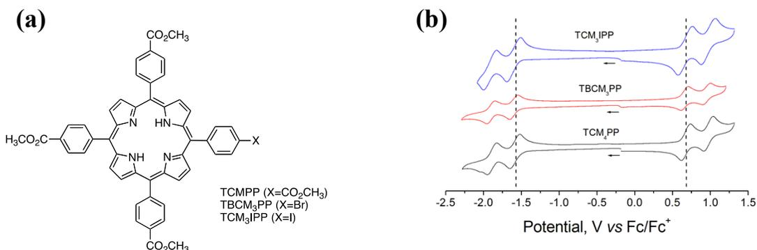
**Figure S1.** (a) Tetraphenylporphyrins synthesized. (b) CV scans of TCM<sub>4</sub>PP, TBCM<sub>3</sub>PP, and TCM<sub>3</sub>IPP in dichloromethane. Scan rate was 100 mV s<sup>-1</sup> with 0.1 M TBAH.
