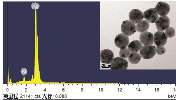
**Figure S1.** EDS image of Ag NPs with a diameter of 35 nm and the inset figure is the TEM image of the synthesized Ag NPs. The EDS image shows that the synthesized Ag NPs consist of pure silver.
