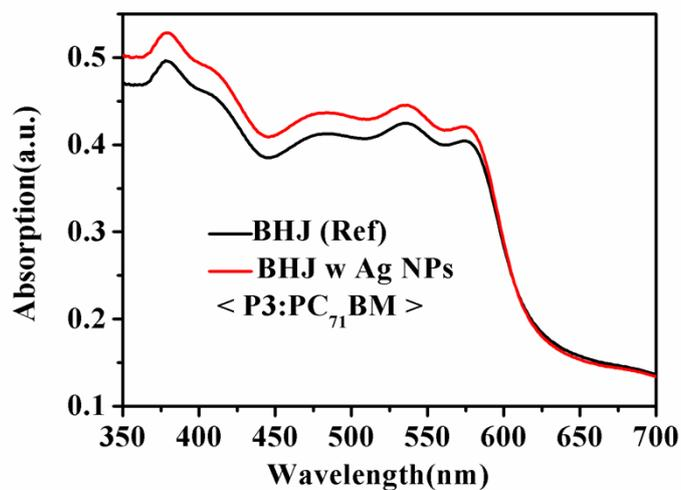
**Figure S2.** UV-vis images of the plain **P1/PC<sub>71</sub>BM** (a) and **P3/PC<sub>71</sub>BM** (b) BHJ films and their BHJ films with Ag NPs with a diameter of 35 nm.
