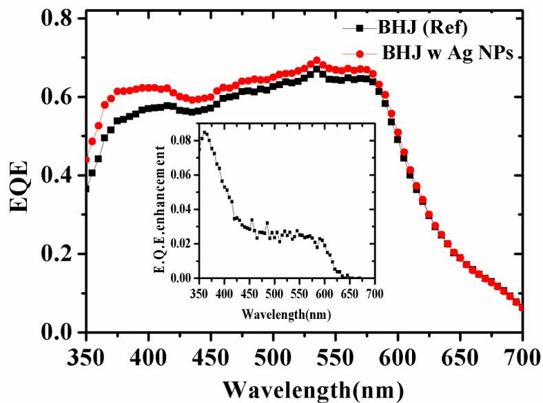
**Figure S4.** EQE spectra of the plain P1/PC<sub>71</sub>BM (a) and P3/PC<sub>71</sub>BM (b) BHJ and the BHJ with Ag NPs. The inset figures show EQE enhancement after incorporating 35 nm-sized Ag NPs into the PSCs .
