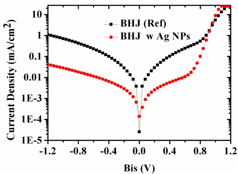
**Figure S5.**  $J$ - $V$  curves of the devices with the plain based on **P1**/PC<sub>71</sub>BM (a) and **P3**/PC<sub>71</sub>BM (b) BHJ and the BHJ with the Ag NPs in the dark current.
