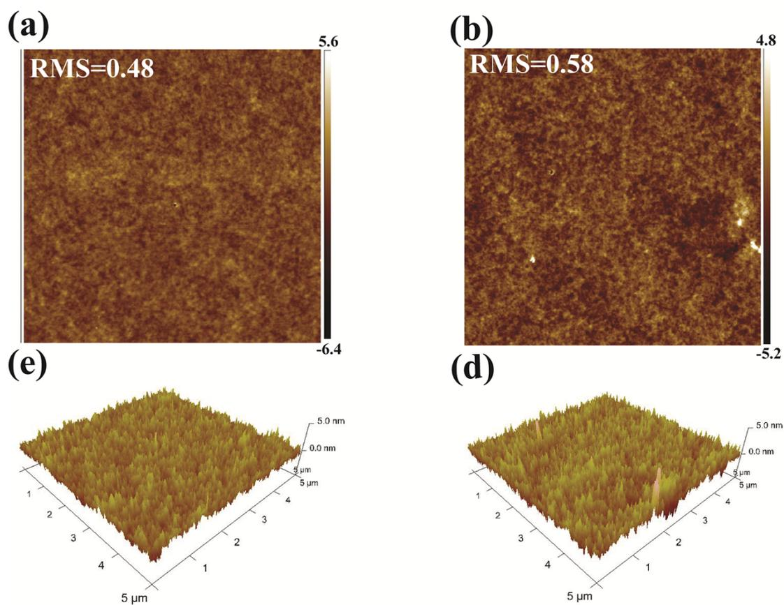
**Figure S3.** AFM 2D height images (left) and 3D height images (right) for **P3/PC<sub>71</sub>BM** active layer on ITO/(Ag NPs)/PEDOT:PSS. The corresponding mean roughnesses (RMS) of these films are 0.48 nm, 0.58nm, respectively. Imaging area: 5
