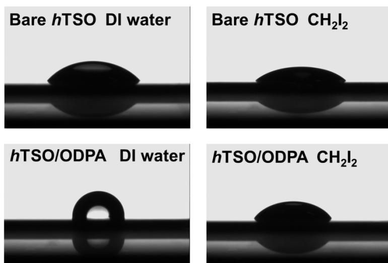
**Fig. S2** (a) DI water and (b) diiodomethane contact angles on *h*TSO and *h*TSO/OPDA dielectric surface.
