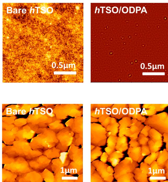
**Fig. S3** AFM height images of (a) the *h*TSO and *h*TSO/OPDA surface and (b) the surface after thermally evaporating 50 nm thick pentacene on *h*TSO and *h*TSO/OPDA.
