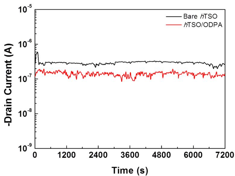
**Fig. S4**  $I_{ON}$  of OTFTs based on *h*TSO and *h*TSO/OPDA dielectric as a function of the time under gate bias stress.
