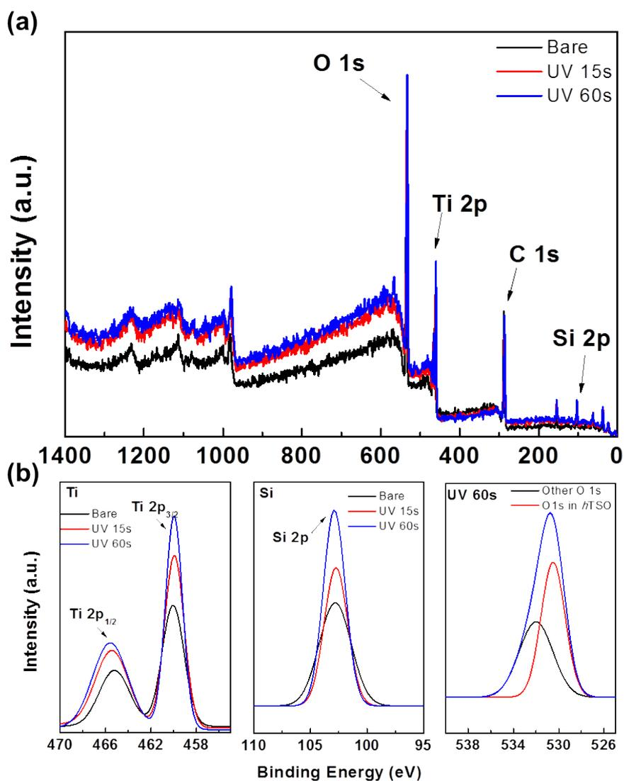
**Fig. S1** (a) X-ray photoelectron spectroscopy (XPS) analysis showing the composition of *h*TSO film. (b) Ti 2p, Si 2p and O 1s core level photoemission spectrum of the *h*TSO film.
