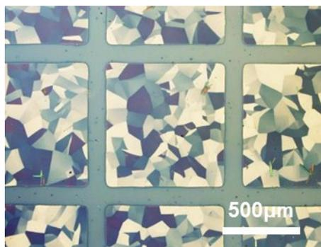
**Figure S4.** POM image of a patterned crystalline rubrene film fabricated on UV-irradiated PS. The thickness of PS is 20 nm.
