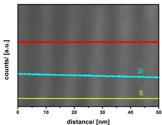
The graphs show a HR-TEM EDX linescan in a high resolution of PEDOT@UKON-2a. The resolution of the EDX measurement is not high enough to reveal the modulation of the silica wall and though the exact distribution of the polymer. Nevertheless a homogeneous distribution of the incorporated polymer and  $\text{FeCl}_3$  is visible.
