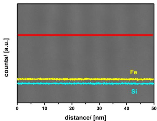
The graphs show a HR-TEM EDX linescan in a high resolution of  $\text{FeCl}_3@UKON-2a$ . The resolution of the EDX measurement is not high enough to reveal the modulation of the silica wall and though the exact distribution of  $\text{FeCl}_3$  in the pores. Nevertheless a homogeneous distribution of the incorporated  $\text{FeCl}_3$  is visible.
