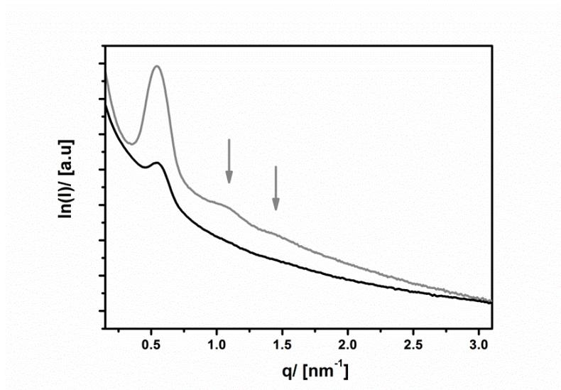
SAXS data of UKON-2a (grey) and PEDOT@UKON-2a (black). Decrease in signal intensity results from the pores being filled up with polymer and developing an electron density similar to the pore walls. However, the position of the main signal at  $q = 0.55 \text{ nm}^{-1}$  remains unchanged.
