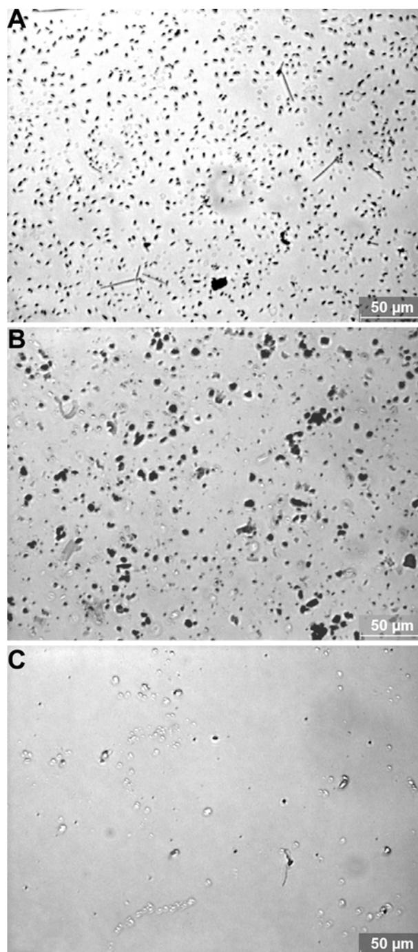
Figure S1. Optical microscopy images of CNMs, (A) CNT, (B) Go and (C) ND.
